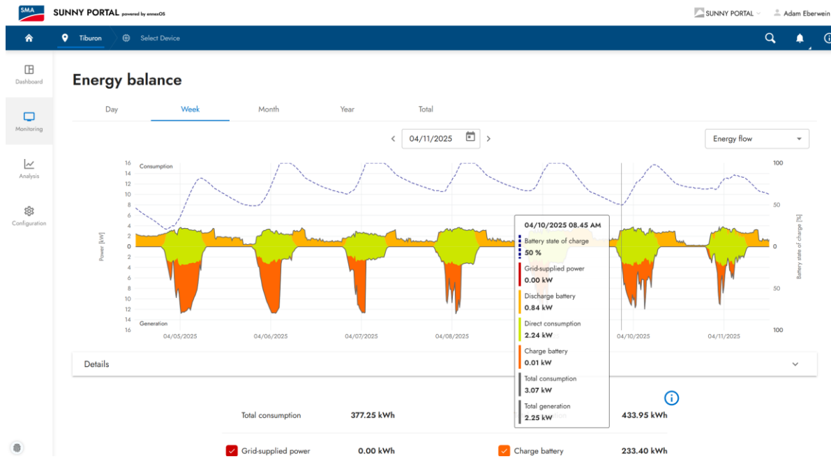
Figure 8: 7-day Tiburon Generation Profile with Example of Solar Clipping
